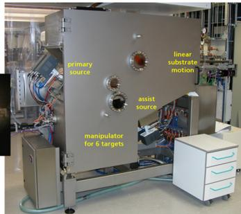
Left hand side: Schematic view of the arrangement for the large-area IBSD. Two linear electron cyclotron resonance ion sources are used for primary sputtering and layer growth assistance or etching.
