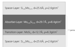
Fig. 3: Structure model of PLD-prepared Mo/Si multilayers.
