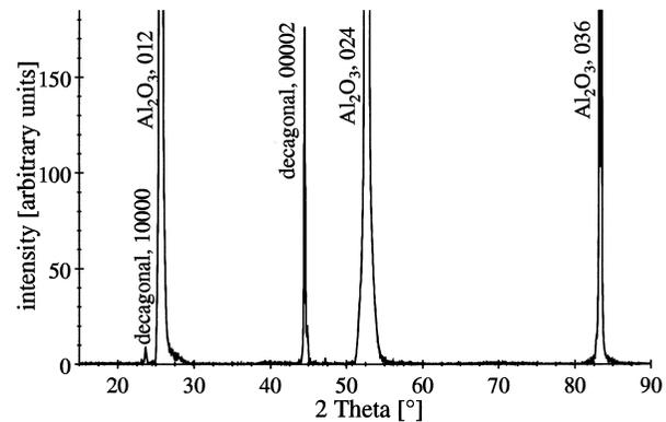
Fig. 4. Diffraction pattern of the symmetrical  $\omega$ - $2\theta$  scan of the quasicrystalline thin film. The sharp and intensive 00002 peak at  $44.6^\circ$  indicates the alignment of the periodic direction perpendicular to the substrate surface.
