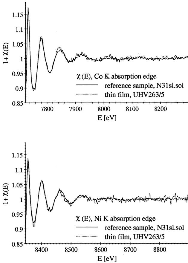
Fig. 5. Comparison of the EXAFS functions of the thin film and of the quasicrystalline reference sample at Co and Ni K absorption edge. High frequency oscillations of solid curve are probably due to the statistics of the small diffraction volume.
