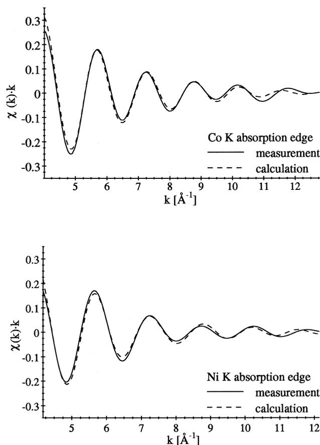
Fig. 6. Comparison of the measured and calculated best fit EXAFS function  $\chi(k) \cdot k$  at the Co and Ni K absorption edge.
