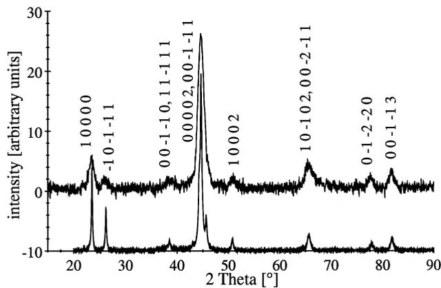
Fig. 3. Diffraction pattern of the quasicrystalline thin film obtained with asymmetrical scan at fixed angle of incidence  $\omega = 2^\circ$ .  $\text{CuK}\alpha$  and a Si-(111) monochromator were used. Indexing according to Kek and Meyer [22]. Long axis of the rectangular sample perpendicular to diffraction plane.
